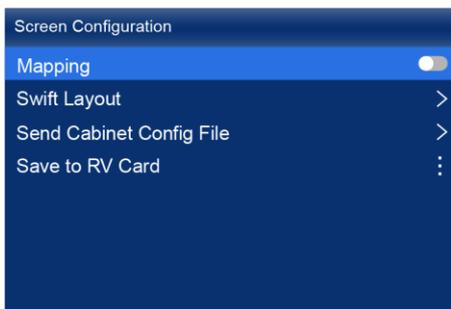
Step 2 Enable the Mapping function by toggling on this switch
