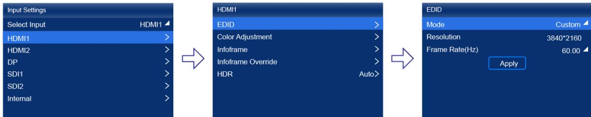
When the device working mode is All-In-One Controller, the **Select Input** menu is not displayed.
