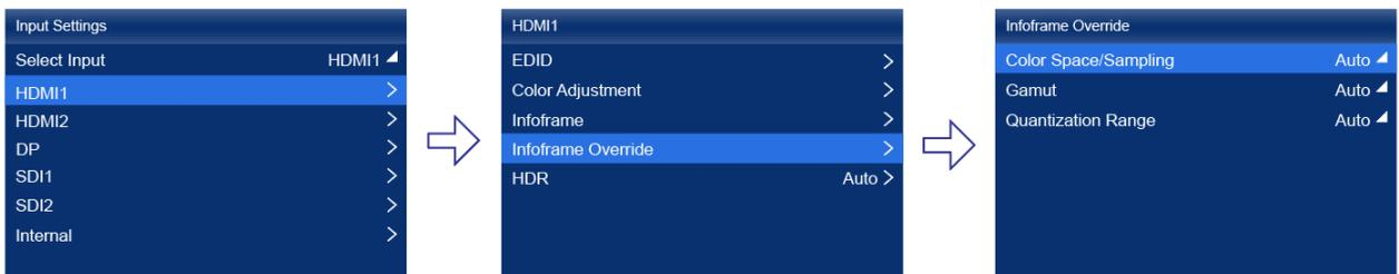
When the device working mode is All-In-One Controller, the **Select Input** menu is not displayed.
